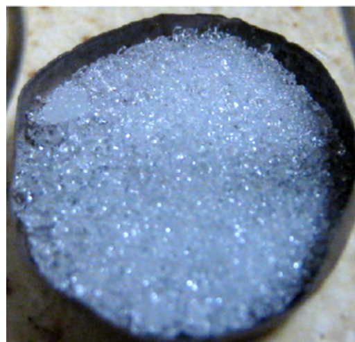
Fig. 8. Typical appearance of a 94%RH sample in a platinum TGA pan, after completing the TGA analysis at 150 °C.
